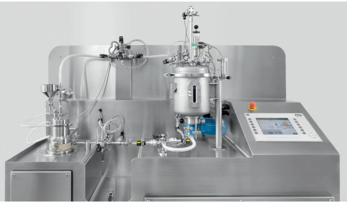
Figure 2 Prototype of nano-milling unit
