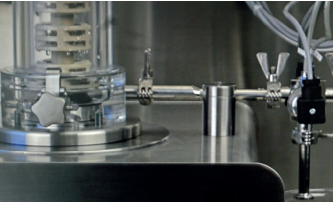
Figure 1 New reverse flow milling chamber
