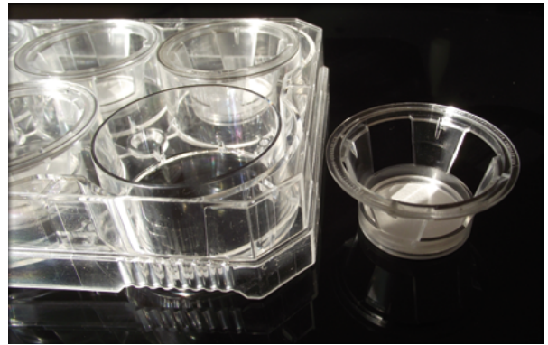
Image 4: Mimetix scaffold in a 6-well format with hanging inserts, allowing exposure to medium above and below
