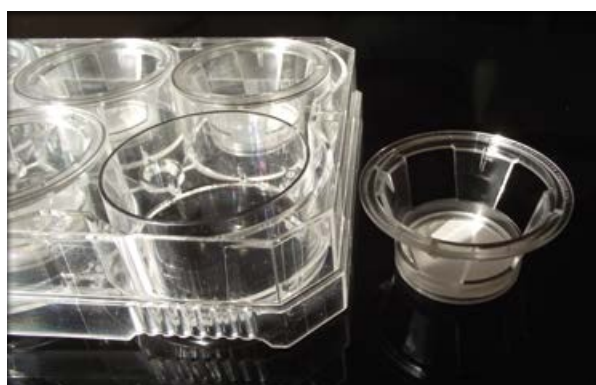
Image 7: Mimetix scaffold in a 6-well format with hanging inserts, allowing the formation of an air-liquid interface which can be used to model tissues such as skin or lung.
