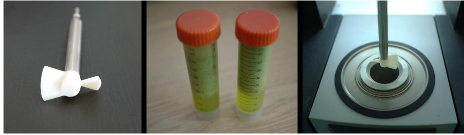
Figure 2 - Photographs showing Kinexus mixing geometry (left), green smoothie displaying separation (middle) and Kinexus with cup and mixer configuration
