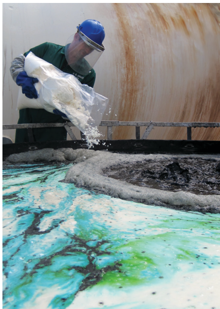
Smopex® 105 being charged into the palladium bearing solution at the customers site.
